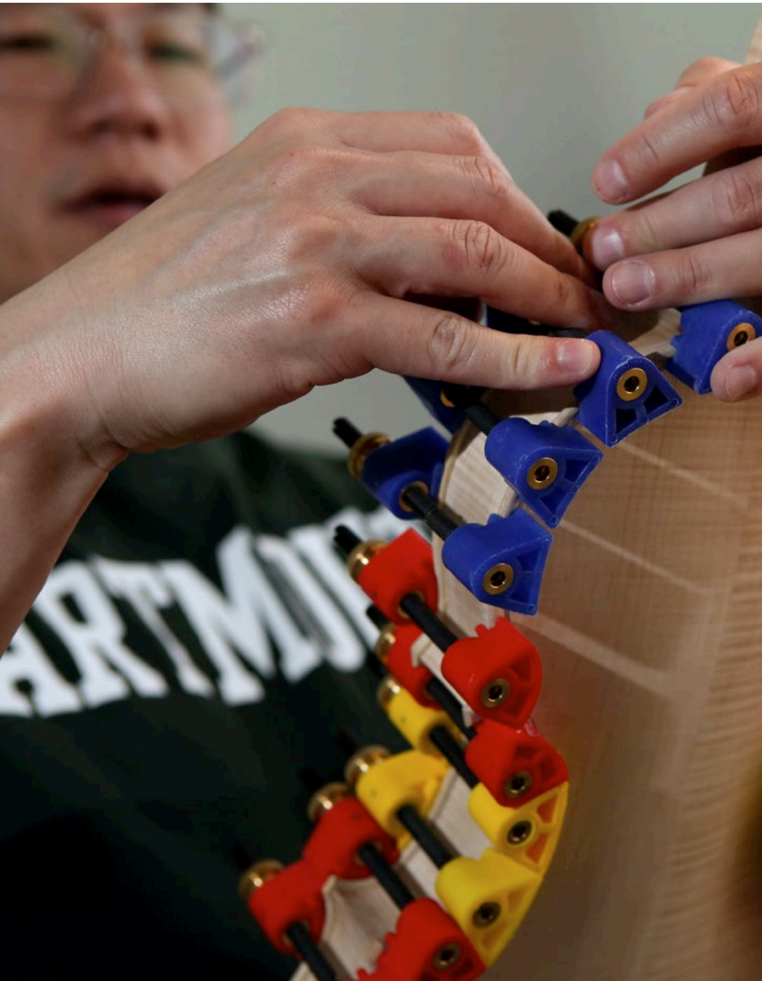
Gluing and clamping top of violin.
