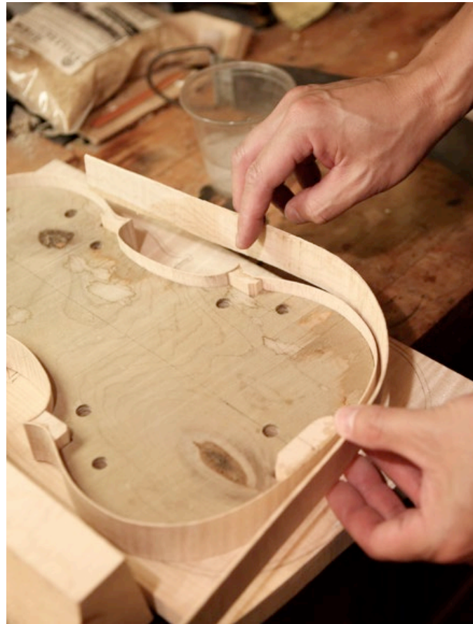
Bending and forming the ribs.
